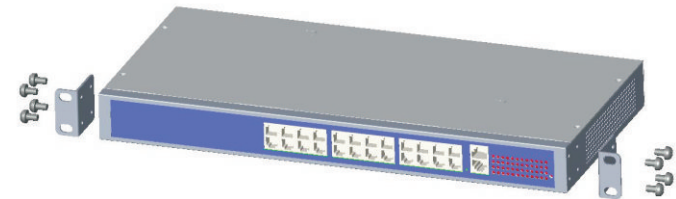
Figure 2-1 Install hangers diagram
