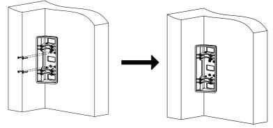
Align the bracket with the wall. Secure the mounting bracket on the wall with 4 SC-KA3X20-NI-JMF screws.
