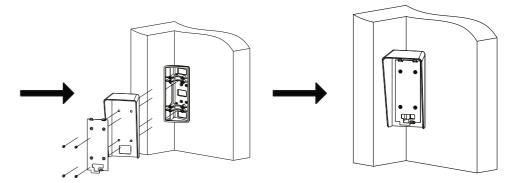
Align the protective shield(DS-KABV6113-RS) and the applied mounting plate with the bracket. Secure the protective shield and the mounting plate on the bracket with 4 SC-KM3X8-BNI screws.
